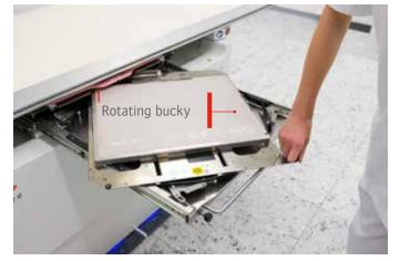
In-bucky detector charger: The fully automated version includes an optional inbucky charger for the detector, ensuring a fast and efficient workflow.
